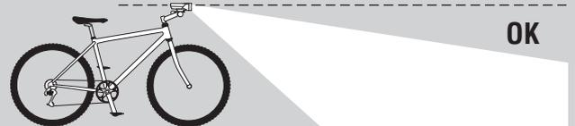
When mounting the light unit, ensure that the light will not dazzle other road users.
